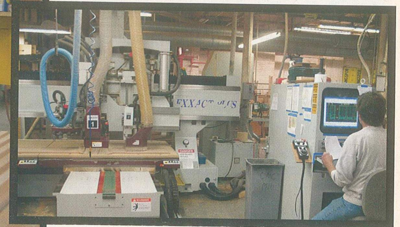
Anderson Exxact Plus dual-table machining center cuts shaped parts such as curved mouldings.
